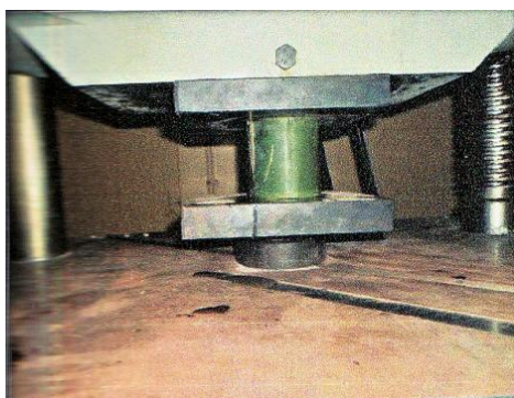
Fig. 2. Compression Test Set-up and typical appearance of specimen at failure
