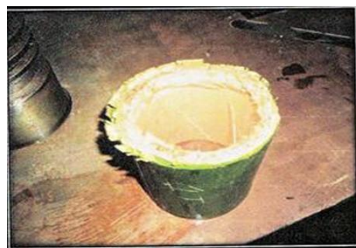
Fig. 2. Compression Test Set-up and typical appearance of specimen at failure
